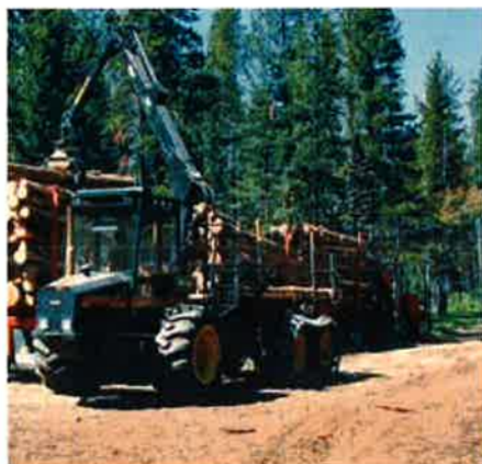
Logs are offloaded from the forwarder directly to log trucks.
