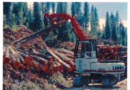
The loader serves two needs: loading trucks and piling tops, branches and log chunks for later burning, chipping or other utilization.
