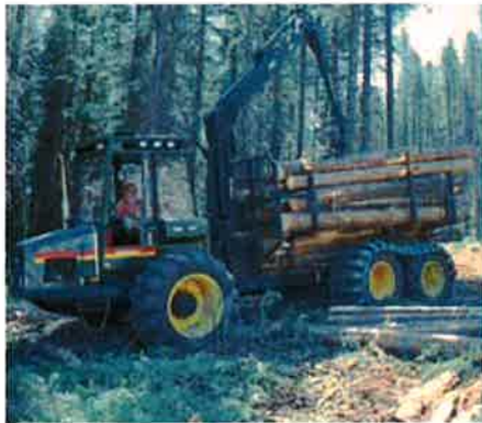
A forwarder follows the harvester, picking up logs and delivering them to log trucks. They can travel long distances, reducing the need for log truck roads.
