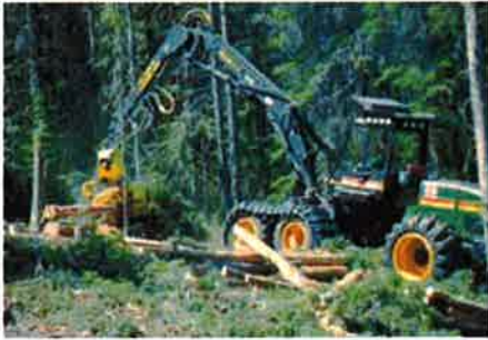
A single grip processor can reach out 30 feet, cut a tree, strip the limbs, cut the stem into pre-programmed lengths and lay the logs on the ground, all in less than a minute. Ideally, they travel over the tree tops and limbs they leave.
